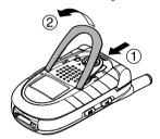
► To install, fit the hooks into the notches on the front of the phone and press down firmly until it snaps into place.
